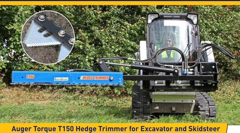
The Auger Torque Hedge Trimmer is the perfect addition for excavators (1.5 – 8T) and skidsteer loaders, and offers a variety of motor sizes to suit your application. Attaching to an excavator provides extra-long cutting reach, gaining access to those taller trees and deeper hedges. The newly designed skidsteer mounting frame allows you to quickly switch the Hedge Trimmer between left and right sides of the skidsteer. The Hedge Trimmer is also ideal for cutting long grass and brush.
